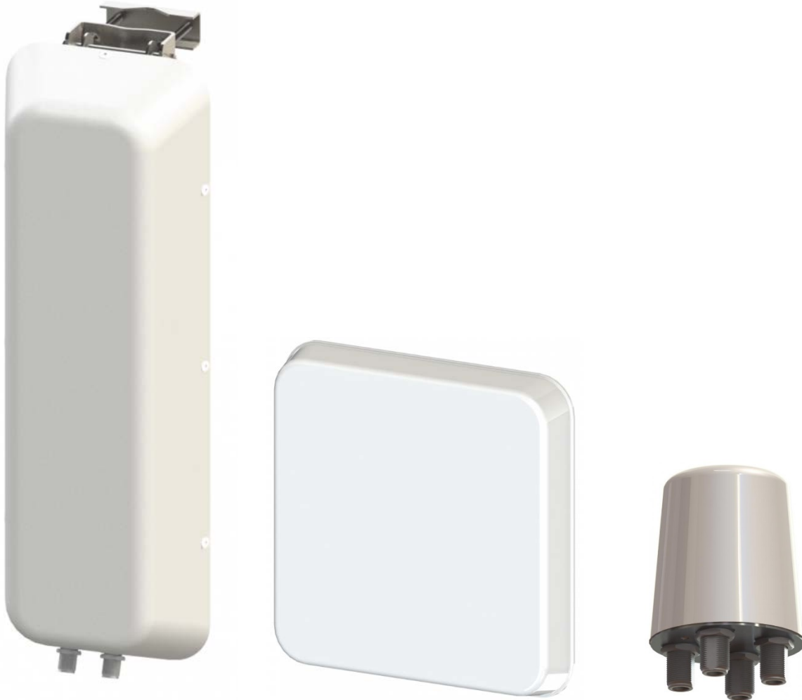
Figure 5: Examples of multi-antenna products designed specifically for MIMO use. Each product features multiple RF connectors, each connected to a discrete antenna within the product's radome. These are often cross-polarized for additional polarization and spatial diversity.
