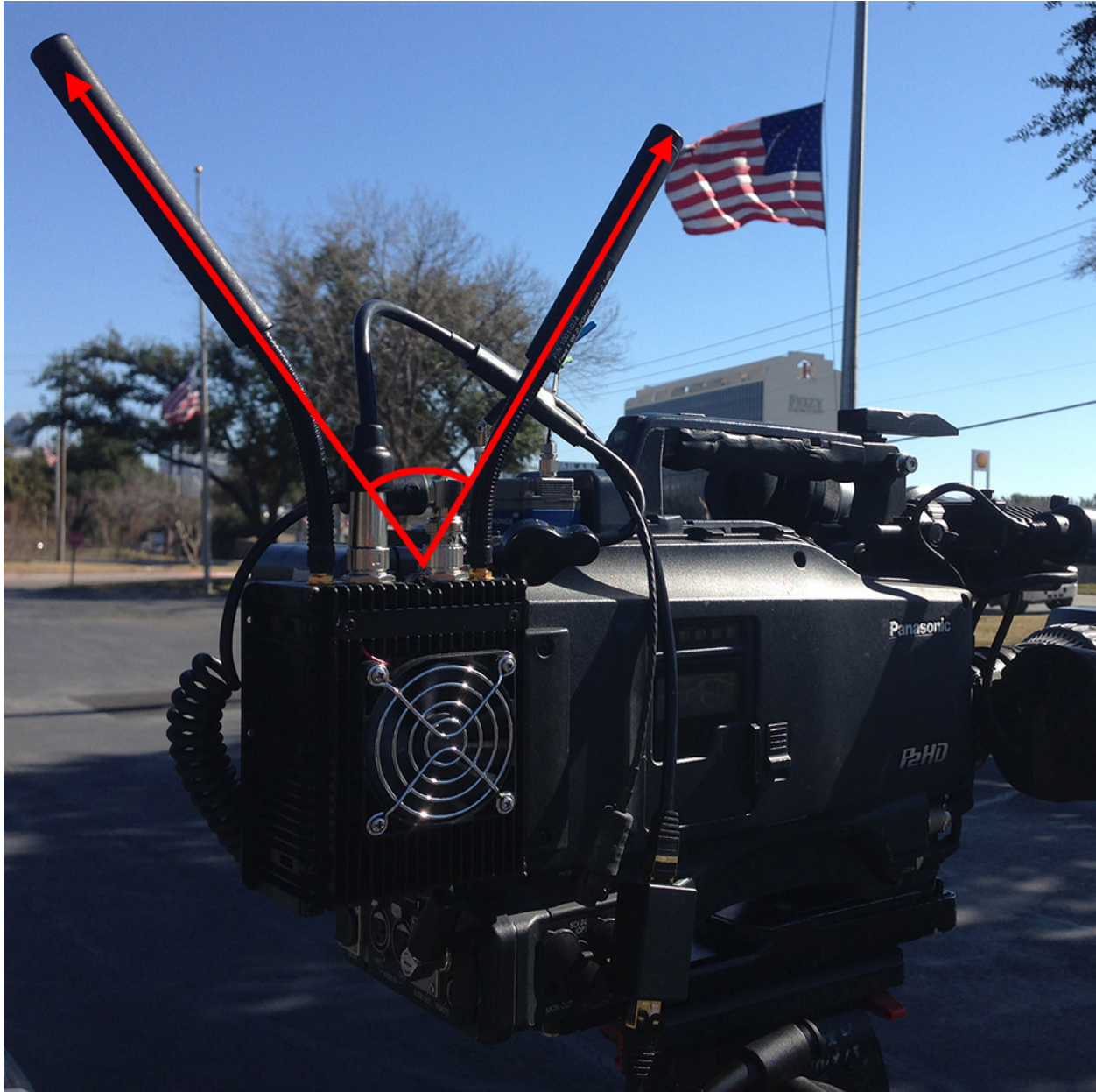
Figure 8: Example of two antennas set at opposite cross-polarized 45 degree angles, offering good polarization diversity.
