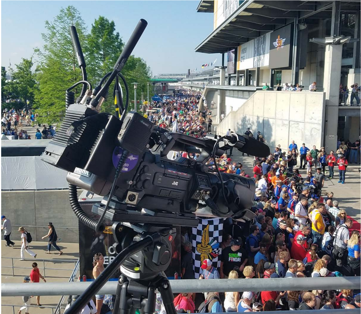
Figure 3: Example of a Silvus MIMO radio with two gooseneck antennas being used to transmit HD video at the Indianapolis 500.
