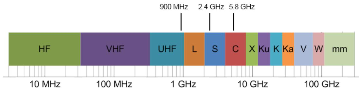
Figure 1: Example of common ISM bands within the IEEE frequency band chart. (Graphic based on "Frequency Band Comparison" by Treinkvist licensed under CC BY-SA 4.0)
