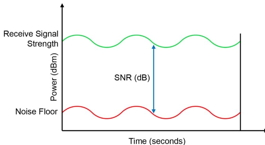
Figure 4: Illustrating Signal-to-noise ratio as the decibel measurement difference between the received signal strength and noise floor.
